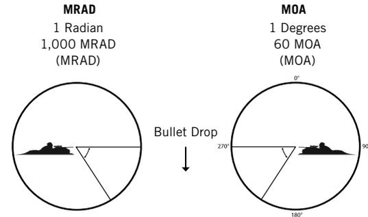
**MRAD** arc measurements are based on the concept of the radian. There are 1,000 milliradians in a radian. A milliradian is always 1/1000th of any unit. So, 1 MRAD is 1m at 1000m, 1 yd. at 1000 yds., or 1 in. at 1000 inches. Most riflescopes using MRAD turrets will adjust in 1/10 MRAD increments. Adjustments can be felt by mechanical “clicks,” which subtend .10 units for each 100 units of distance (e.g. 0.1 yd. or 0.36" at 100 yds.; 0.2 yd. or 0.72" at 200 yds.; or 1cm at 100m, 2cm at 200m).
