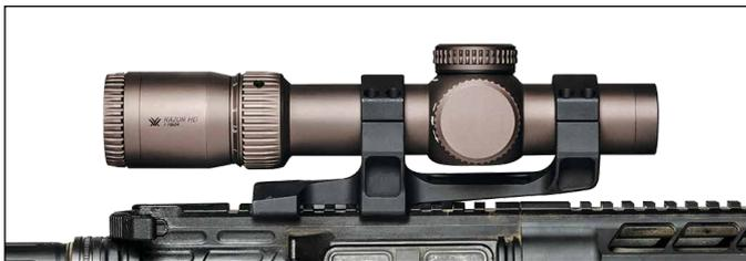
**NOTE:** Vortex Optics recommends not exceeding 18 in./lbs. of torque on the ring screws, and not exceeding 35 in./lbs. on the base screws. If using something other than a Vortex® mount, verify torque from manufacturer specifications. **DO NOT** use a thread locking compound on the threads. Thread locking agents lubricate the threads, which can increase the applied torque. If thread locker is used on the threads, do not exceed 11 in./lbs. on the ring screws.
