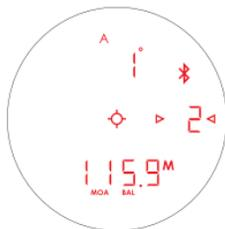
This number is automatically calculated into the wind/drop solution provided in the display and in the GeoBallistics® App. If you are not using the on-board solver, enter the slope incline number into ballistic programs or field cards to help calculate precise bullet drop in mountainous terrain. To use the Razor® HD 4000 GB on-board ballistic solver, you need to be in BAL Mode.
