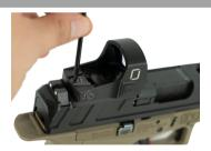
Use a flathead key to make elevation adjustments to your red dot's position. As indicated, counter-clockwise moves your Point of Impact UP. 1 Click = 1 MOA
