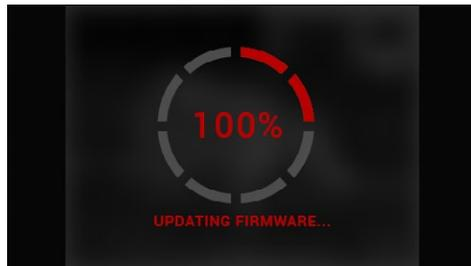
10. Please delete the Firmware file off of the microSD card after the process is complete. Or the system will try to update the Firmware every time you turn the scope on.
