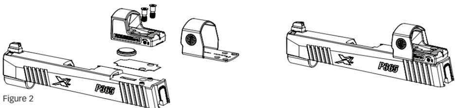
**INSTALLING AND CHANGING THE BATTERY:** The ROMEOZero must be removed from the firearm to access the battery. The CR1632 coin cell battery is installed from underneath the sight. Insert the battery into the round battery slot with the positive (+) side facing out, toward the pistol slide, and temporarily hold it in place using a thumb or finger until you're ready to mount the sight onto the firearm.
