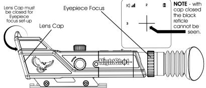
Set Eyepiece Focus once only. **Do not readjust** unless a different shooter uses the scope.
