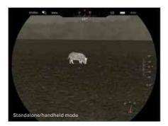
The MICRO also features use specific display modes for handheld, helmet mount, direct view or clip-on operation. When transitioning from handheld use to helmet mounted use, the display will automatically change accordingly. This incredible versatility is taken one step further with the iRayUSA PICTAIL system and its innovative combination of industry standard dovetail and picatinny mounting solutions. Learn more about the RICO MICRO by visiting irayusa.com/rh25.
