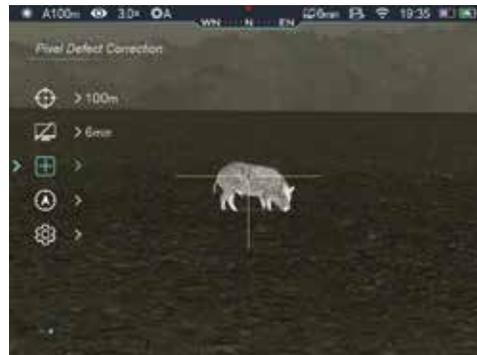
Rotate the controller turret (7) to move the cursor to align with the defective pixel.
