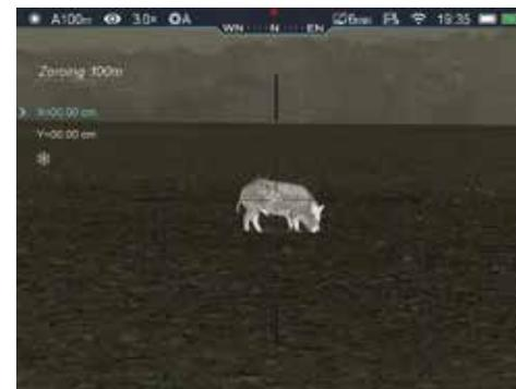
If the impact point does not match the aiming point (the center of the reticle), keep the reticle centered on the aiming point, then press and hold down the Palette Button (6) and Photo Button (3) at the same time until a freeze symbol ❄ appears on the left of the screen, and the image is frozen.
