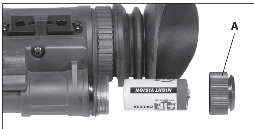
Figure 4.1 CR123A Battery Installation
