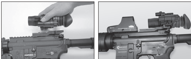
Figure 3.3 Attaching ATN NVM-14 to Weapon Mount
